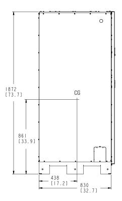
Figure 3-8. ISBM Section Center of Gravity
